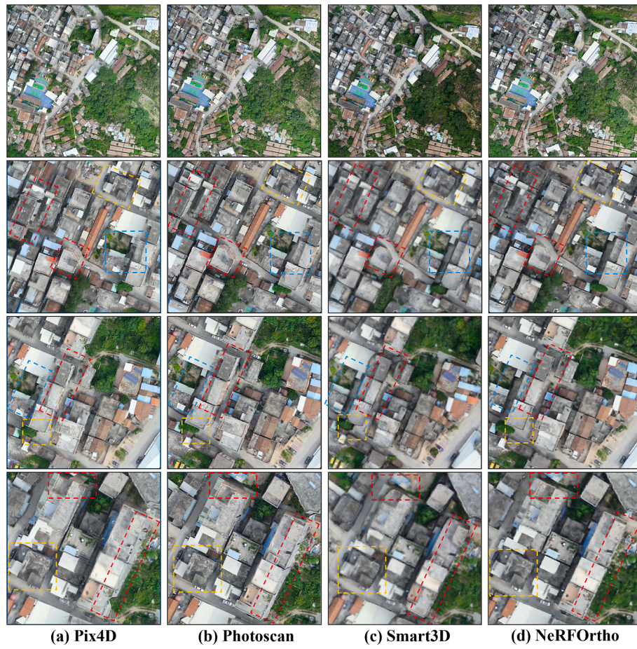
Fig. 8. Comparison of TDOM generated with software Pix4D, Photoscan, and Smart3D with NeRFOrtho in real UAV data.
