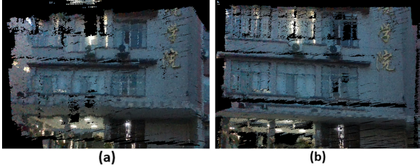
Fig. 14. The calibration result of our Velodyne VLP-16 LiDAR devices: (a) coarse calibration (b) fine calibration.
