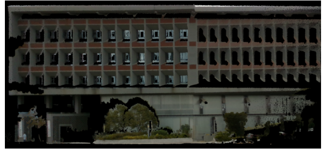
Fig. 1. Point cloud accumulated by a Livox Avia LiDAR. It is colored using an image and extrinsic parameters generated from the proposed method. The color detail of the point cloud has been restored correctly.
