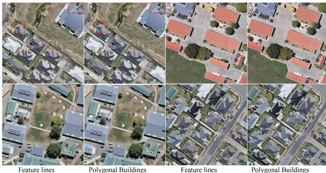
Fig. 12. Examples of feature line and polygonal building results achieved by Line2Poly on the WHU aerial building dataset. The left side of each group of images shows the feature line extraction result, and the right side displays the building polygon reconstruction result.
