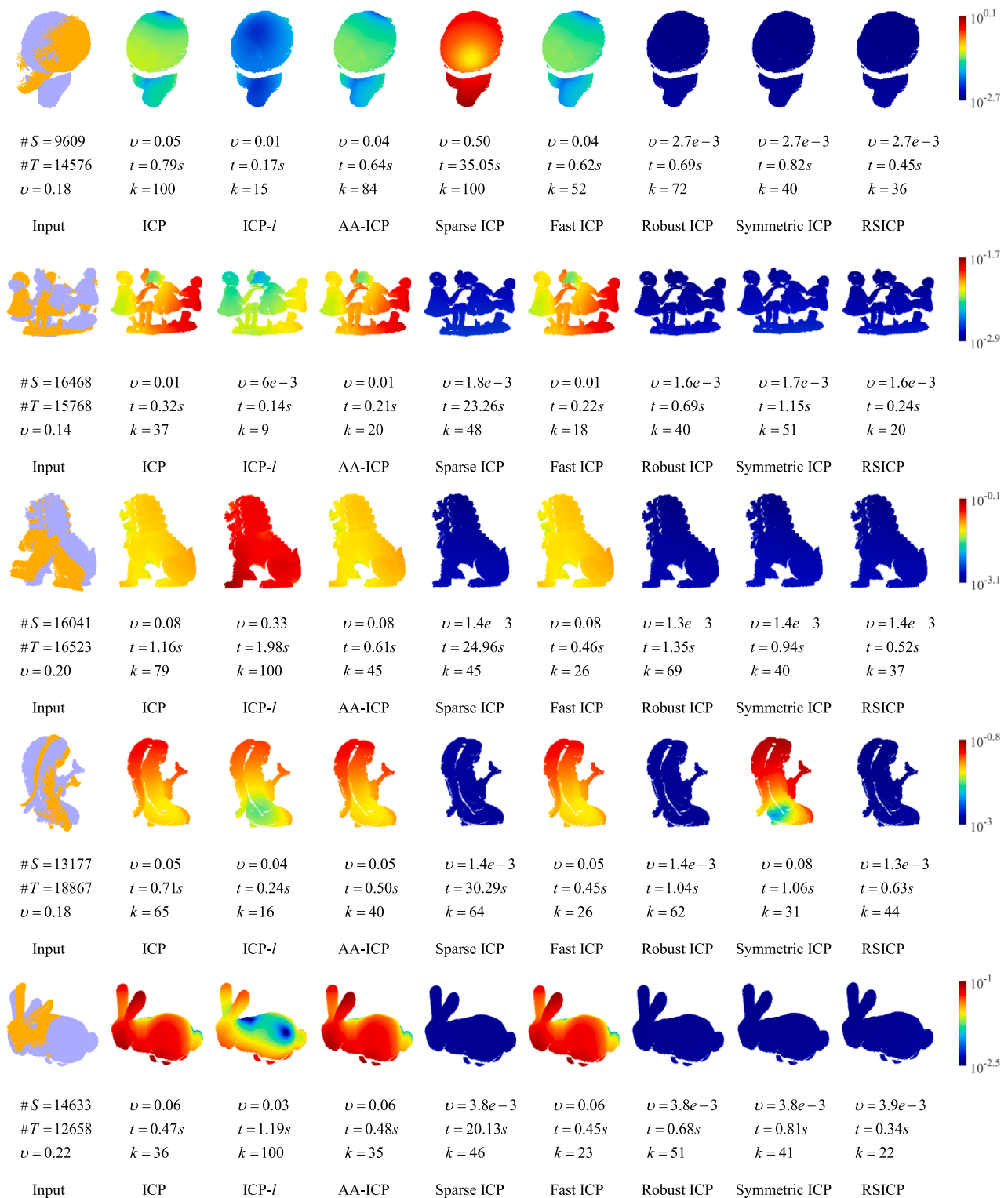
Fig. 6. Registration results on several example instances of the FGR dataset with partial overlaps. The registration RMSE, running time, and iteration number are reported below each result, where the RMSE is reflected by the error map using log-scale color-coding.
