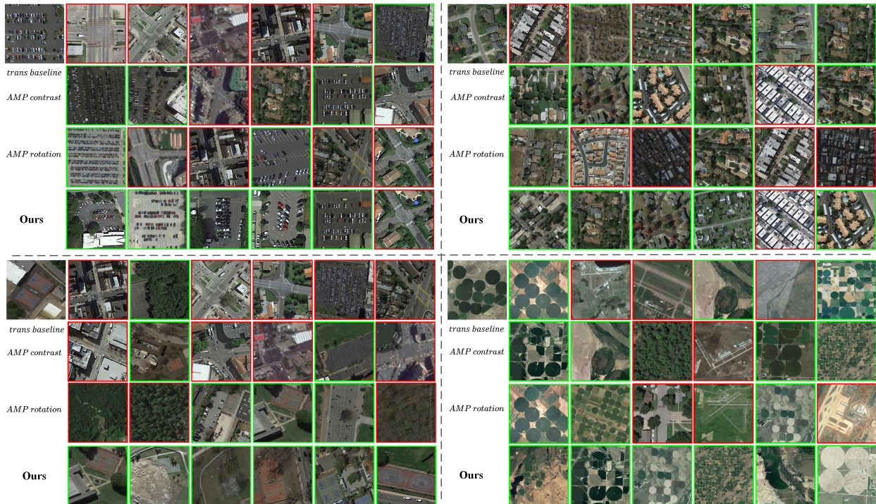
Fig. 6. Nearest-neighbor retrieval results. We show the six nearest neighbors of trans baseline , AMP contrast , AMP rotation , and our method. Queries are randomly selected from novel classes of NWPU-RESISC45. The semantic labels of the four queries are “parking lot,” “medium residential,” “basketball ground field,” and “circular farmland,” respectively. Semantically related and unrelated retrievals are separately marked with green and red boxes, respectively.
