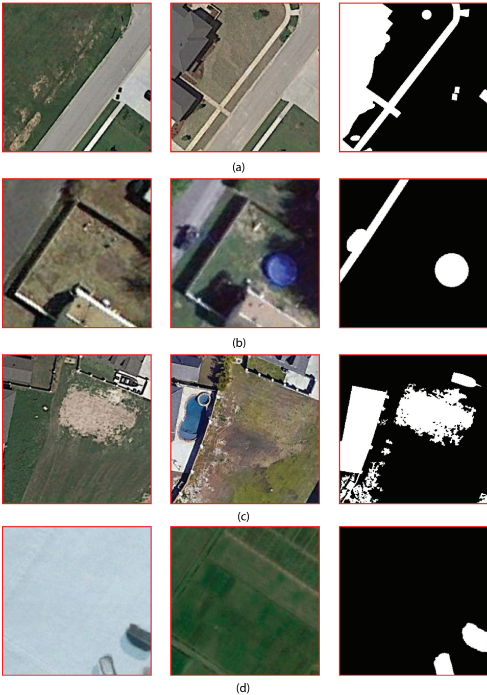
Figure 4. Example samples of the VHR dataset (Lebedev et al. 2018). In each line, from left to right, are image T_1 , image T_2 , and the labeled change map. The examples include the changes in buildings, roads, cars, and the not considered season-varying scenario.
