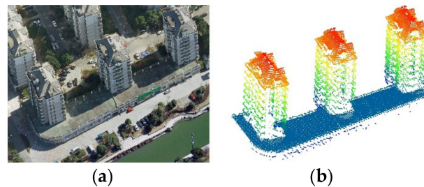
Figure 3. Podium building: (a) aerial image corresponding to podium buildings; (b) podium building point clouds.
