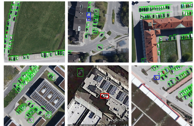
Fig. 7. Examples of detection results of our method on Munich dataset. Green boxes indicate the correctly detected vehicles, blue and red boxes indicate the missing and false alarms respectively.
