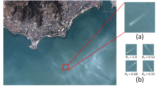
Fig. 8. One frame of the satellite video we use for experiments. (a) The fishing boat we used for tracking. (b) The multi-angle templates and corresponding matching results.
