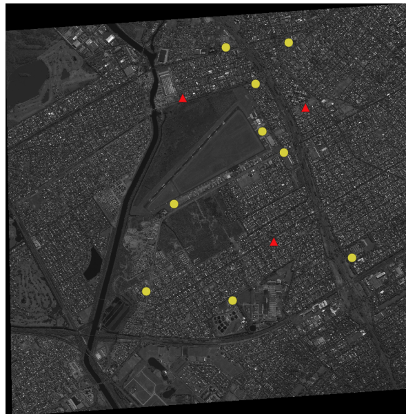
Figure 10. The distribution of 12 ground control points (GCPs). 3 GCPs marked with red triangles were applied in the BA process while other GCPs marked with yellow circles were used to check the accuracy of the BA result in the object space.
