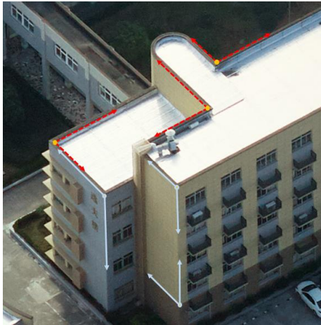
Figure 2. The L-junctions in white solid lines can be used to extract planes, while those in red dash lines cannot.
