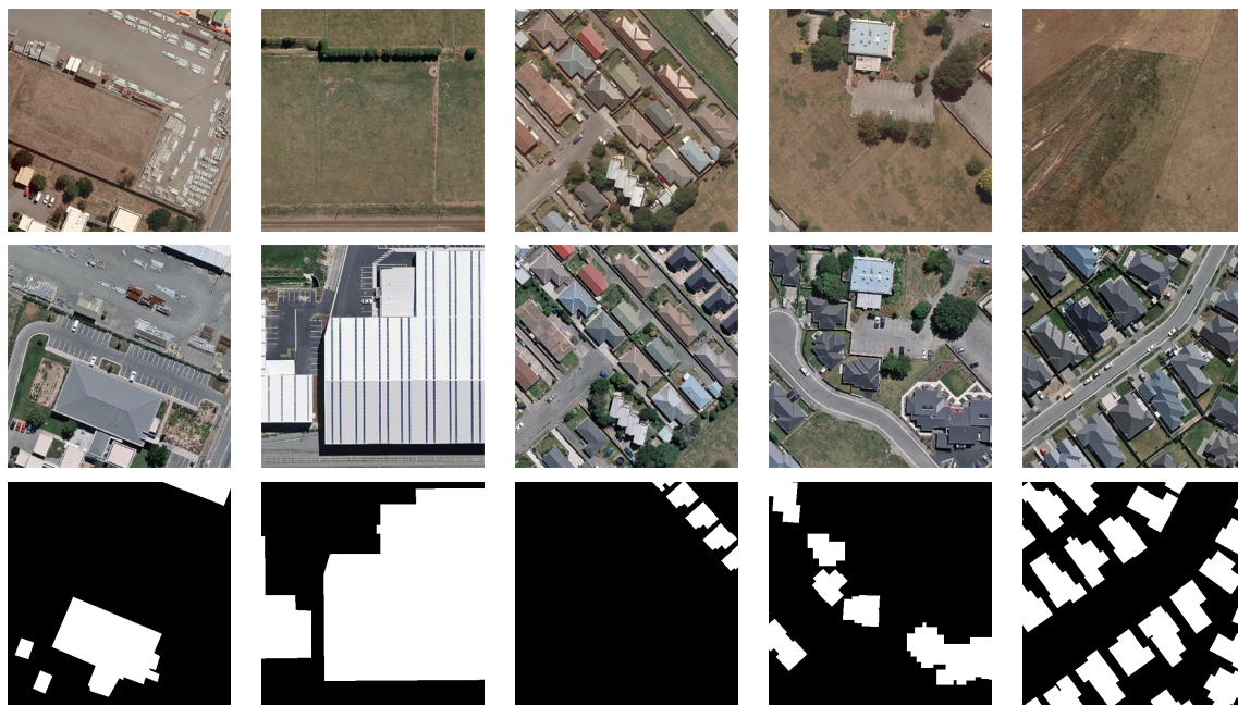
Figure 8. Examples of changed buildings. The top row is images of 2011, middle row is images of 2016 and bottom row is the change labels.
