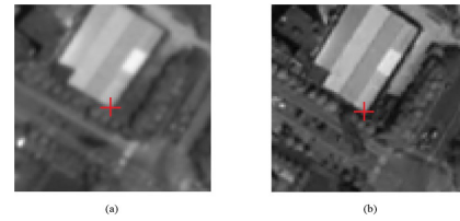
Fig. 4. Example of checkpoint on the (a) reference image and its projection point on the (b) SRNE fine registered image.
