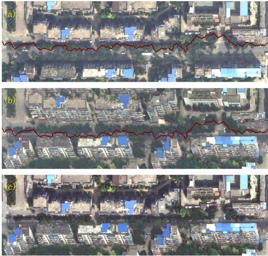
Fig. 14. Sub area A1, showing details of refined seam determined using the proposed method: (a) upper image overlapping refined seam, (b) lower image overlapping refined seam, and (c) mosaicking result without feathering.
