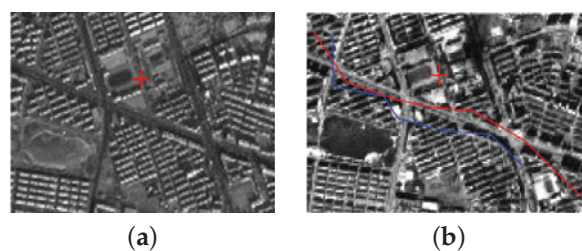
Figure 6. Epipolar lines generated by GC^3 and the developed method: (a) a checkpoint on the test image; (b) zoomed view of epipolar lines; the red one is generated by the developed method, and the blue one is generated by GC^3 .
