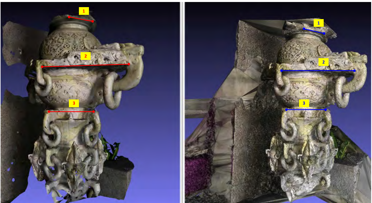
Fig. 13 Measurements in 3D model of the statue 1, left image shows the 3D model reconstructed by our method, right image shows the 3D model reconstructed by Pix4D
