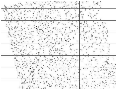
图 8 卫星影像匹配矢量描述子分布示意图 Fig.8 Distribution of vector descriptors in satellite image matching results
