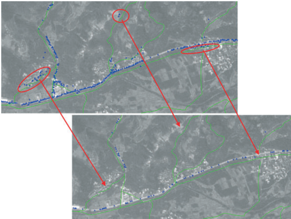
FIG. 7. Road centre point extraction results. Top: without constraints. Bottom: with constraints. Green lines indicate the initial projected roads; blue crosses indicate the extracted road centre points.
