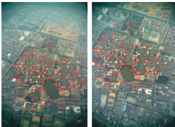
FIG. 11. Matched conjugate points by SIFT operator of a stereopair with 15-degree roll angle.
