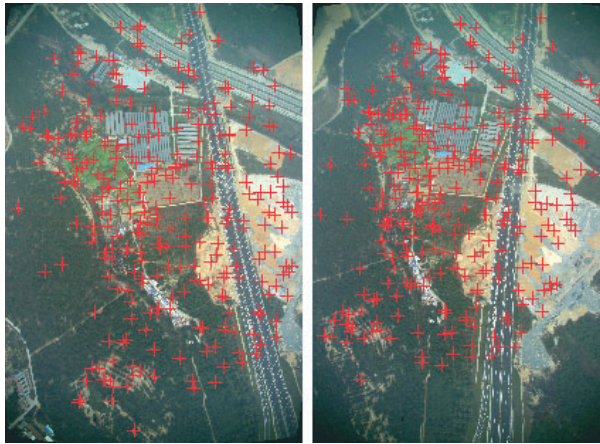
FIG. 12. Matched conjugate points by SIFT operator of a stereopair with 8-degree roll and 22-degree yaw angle.
