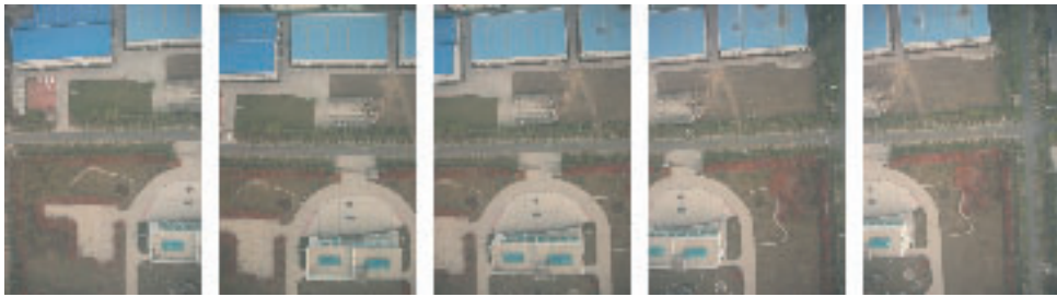
FIG. 4. Stereo-images of the North testfield taken by the airship-borne system.
