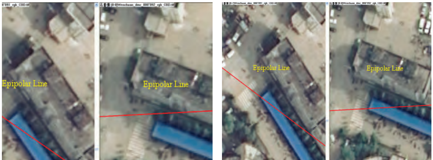
Figure 4. Y-parallax before (left pair) and after (right pair) POS supported bundle adjustment.
