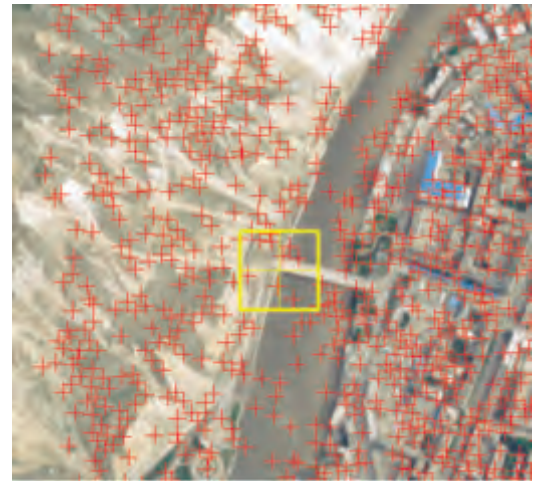
Figure 3. Stereo matching results of images with a 30^\circ rotation angle.
