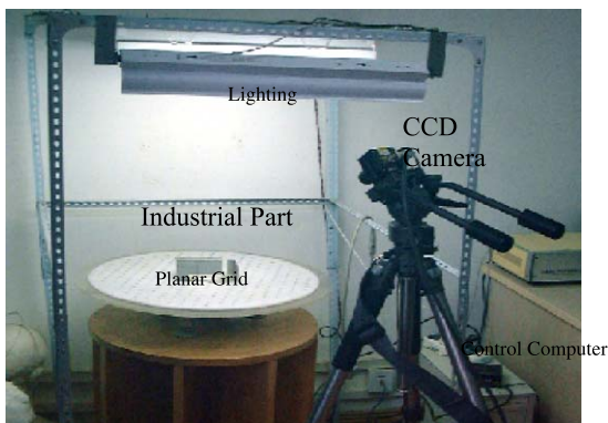
Fig. 9. Hardware configuration of the measurement system.
