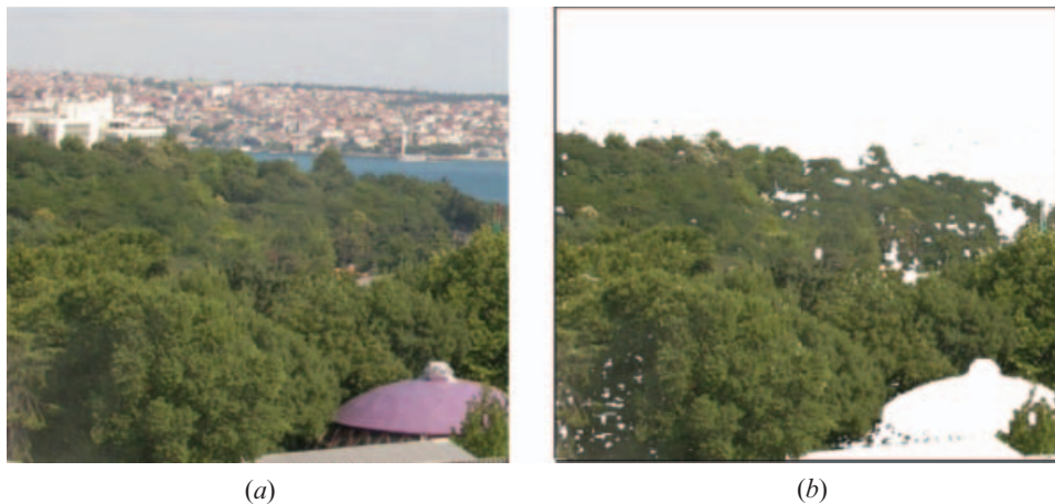
Figure 8. (a) RGB image (Istanbul, Turkey) and (b) result of segmentation by CIE L^*a^*b^* .
