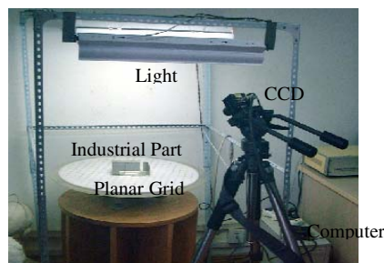
Fig. 8. Hardware of the inspection system Fig. 9. One image of the part to be inspected
