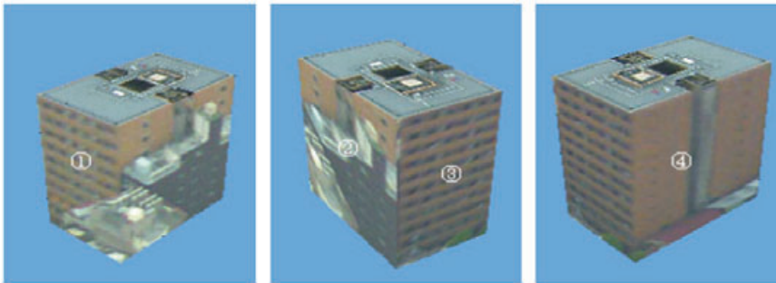
FIG. 8. Textures of walls occluded by other buildings.
