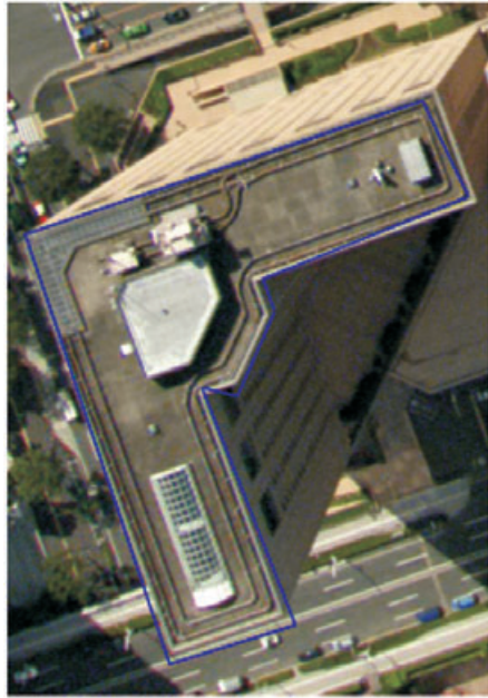
FIG. 4. Imprecision of 2D vector data.
