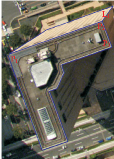
FIG. 5. Matched image lines of a building.
